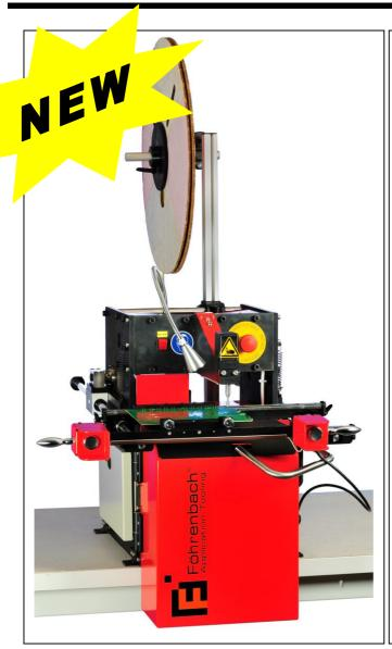
PPY23077 is Föhrenbach Application Tooling newest manual pin insertion machine. The machine accepts contacts that are mounted on a bandoleer. The contacts can feature a solid- or flexible press-fit zone.
