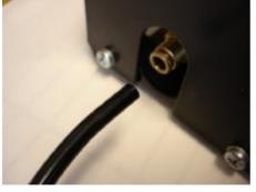
Connect the foot pedal to the crimping tool
