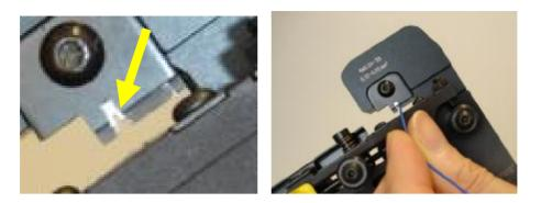
Whilst keeping carefully the wire in position, close the handles until the ratchet releases.
