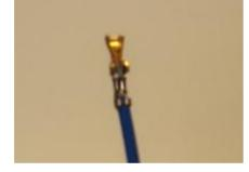
The tool is not cutting the carrier strip. In order to work properly, the operator has to cut the carrier strip on a regular base.
