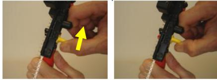
Feed a terminal into the crimping area of the hand tool.
