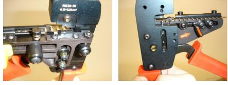
As shown on the picture, insert the strands of a stripped and straightened wire into the slot of the wire positioner. The insulation of the wire should be pouched to the surface of the wire positioner.
