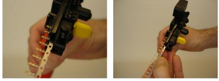
Once 50 mm of the contact strip is introduced into the terminal guide, the contacts can be fed one by one towards the crimp area. In order to do so, activate the manual feeder as shown on the pictures.
