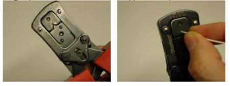
Keep the wire fixed in position and activate the levers till they reach the end position.
