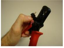
Push the locator towards the crimping die. A magnet will keep the locator in position.
