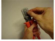
Release the levers and pull out the crimped contact.
