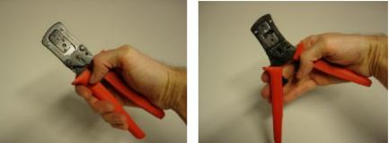
Pull the locator in its 'load position'.
