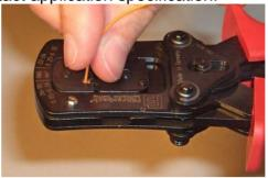
Keep the wire fixed in position and activate the levers till they reach the end position.
