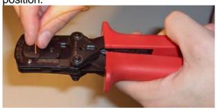
Release the levers and pull out the crimped contact.
