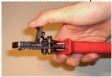
Introduce the contact. Push the contact till it reaches the hard stop.
